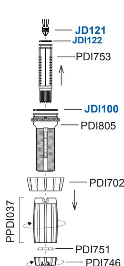
Reinstall "C" clamp by sliding it gently over the thread at the bottom of the white stem. Rotate clamp until it clicks into place.
