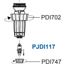
7. Push complete injection stem assembly in position at the bottom of the blue body, making sure desired scale is facing front of injector. Keys at the top of the black sleeve should slide into the slots at the bottom of the body. Slide injection stem nut (PDI702) up the sleeve and screw back on. Insert hose back onto the bottom of the check valve barb (PJDI117). Screw hose nut (PDI803) back on.
